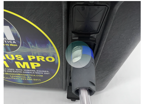
Press into the socket
